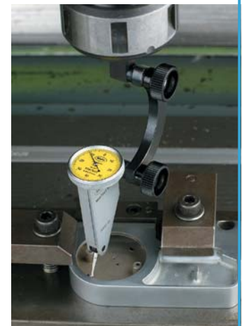
Centering of a bore
