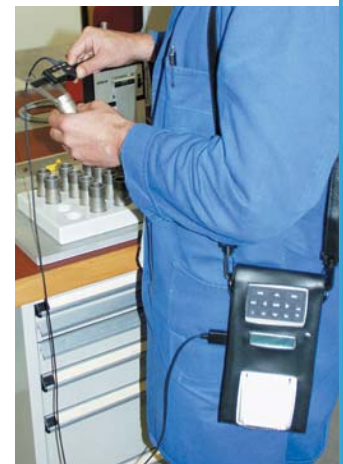
Above shows the Statistics Printer MSP2 being used in conjunction with the Transport Bag MSP 2t
